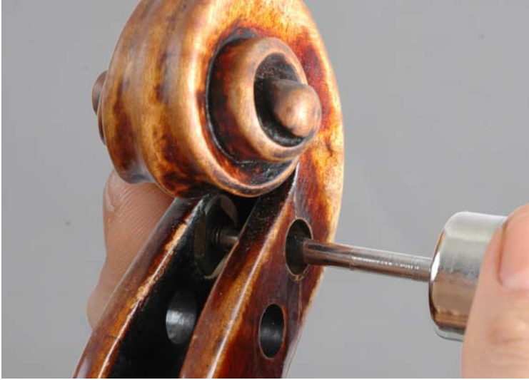
Fig. 4 Cutting the hole
