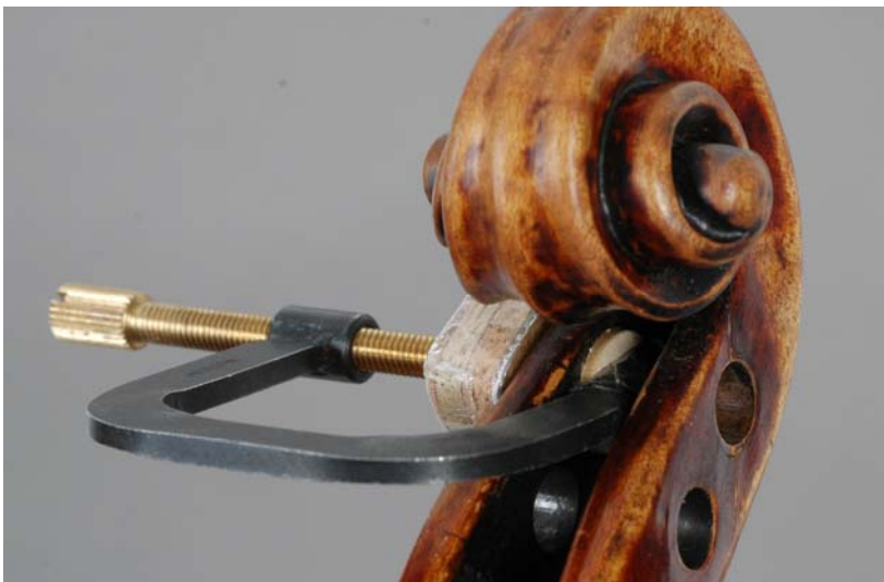
Fig. 6 Gluing the conical bushing
