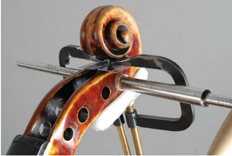
Fig. 7 Gluing the shaving
